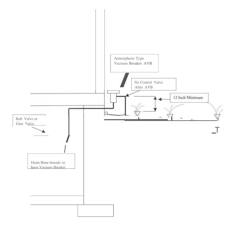
Atmospheric Vacuum Breaker on lawn sprinkler system must be installed at least 12 inches above highest sprinkler outlet and on the non-pressure side of the last control valve.
