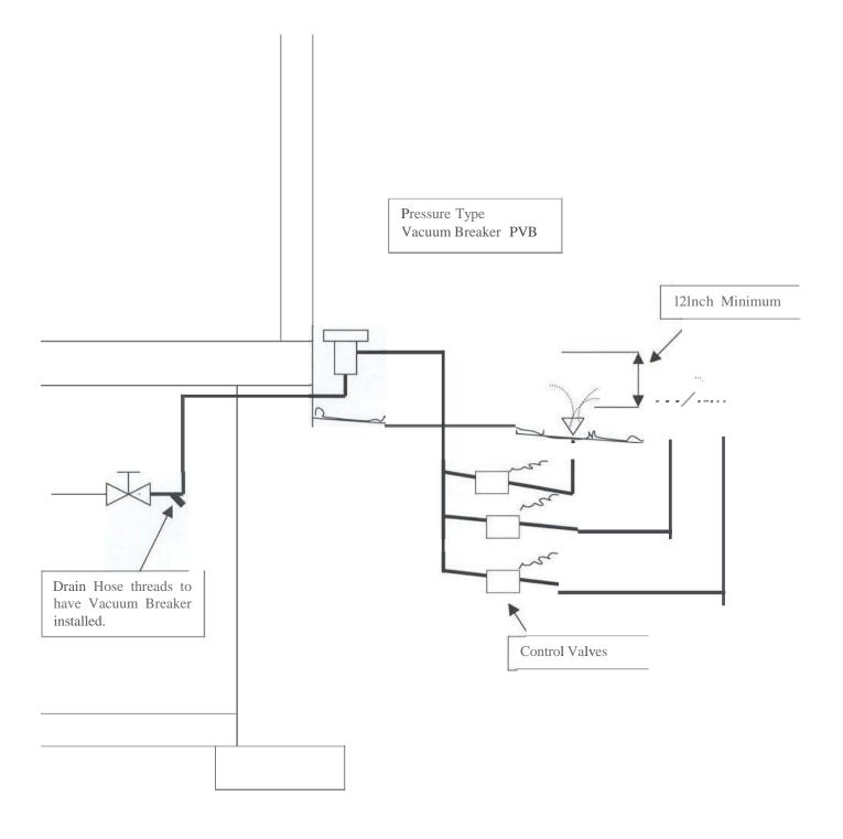
Pressure Vacuum Breaker on lawn sprinkler system must be installed at least 12 inches above highest sprinkler outlet and may be subject to constant static pressure. Note: Per MN Plumbing Code Parts 603.5.23 through 603.5.23.4, the backflow prevention device must be inspected every year by a certified tester or licensed plumber.
